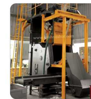
Loader Cabinet & Belt Conveyor
