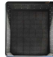
Blast Chamber Manganese lining
