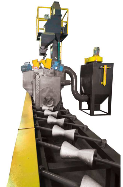
Diabola Conveyor & Dust Collector System
