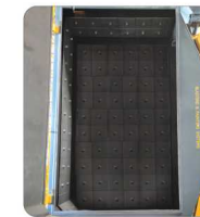
Blast Chamber Manganese Lining
